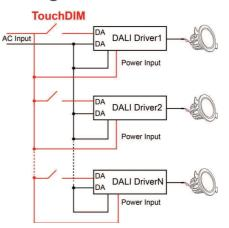
Remark: Only use open push button without indicator light. Maximum cable length between each Unit: 20 meters.
