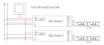
Remark: Only use open push button without indicator light. Maximum cable length between each Unit: 20 meters.
