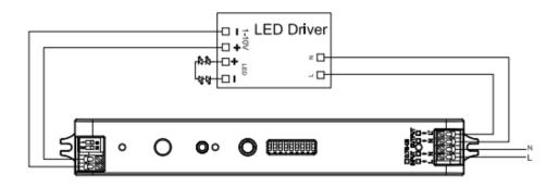
\*The sensor is designed for connect one load only. Connect more than one loads may damage the sensor.
