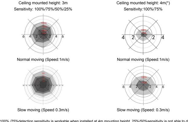
\*Only 100% /75% detection sensitivity is workable when installed at 4m mounting height. 25%/50% sensitivity is not able to detect motion signal.
