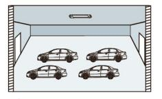
With sufficient ambient light, the light will not be switched on even if with motion signal.
